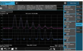
▲ Fig. 1 A single press on the menu panel provides direct access to capabilities such as Keysight's Noise Floor Extension (NFE) technology, which yields an improvement of up to 12 dB in the spectrum analysis noise floor.
