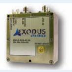
he EDPLO-4000 series phase-locked dielectric resonator oscillator (PLDRO) from Exodus Dynamics externally locks to a 10 MHz reference to achieve crystal stability up to millimeter wave frequencies. Frequency coverage is from 30 MHz to 50 GHz, and the low profile and rugged construction of the RoHS-compliant design provides excellent durability against harsh environments due to shock, vibration, temperature and humidity.
