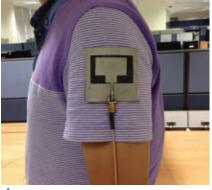
📤 Fig. 2 Arm-mounted wearable antenna.
