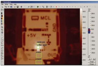
Fig. 4 Thermal image to determine case, PCB, ground lug and MMIC body temperature.
