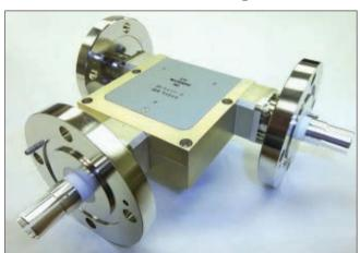
Model CT-1864-S is rated at 60kW peak and 600W average power at 325 MHz. The unit provides 20 dB minimum isolation, 0.2 dB insertion loss and 1.20:1 maximum VSWR. Its extremely compact design has flange to flange insertion length of only 6-3/4" and a height of 5-1/4". For use in radar applications, it has 1-5/8" EIA connectors. It is also available at other UHF frequencies and connector types.
